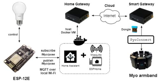
Fig. 1: The presented EMG-based IoT system architecture
