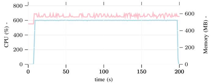
Fig. 7: YOLOX ROS 2 node activity during the mission where CPU usage is shown in blue and memory in pink (100% CPU / processor core).
