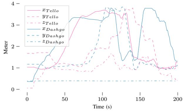
Fig. 4: Trajectory components for each of the robots. At the end of the mission, the robot trajectories converge as the Tello docks on top of the Dashgo.
